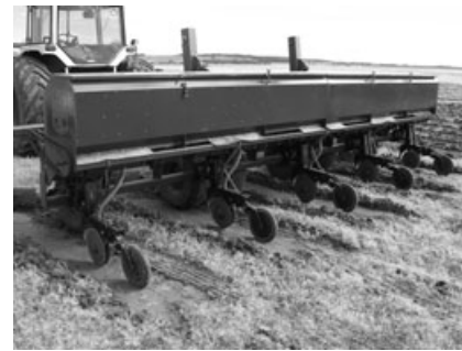
Figure 6. Agricultural precision placement seeder modified for sowing local native woody plants at Peniup. The design builds on a long history of direct seeding equipment development, influenced by many sources.
