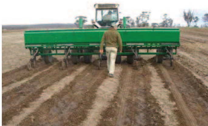
A newly developed five-row direct-seeding machine minimises soil displacement, and reduces row spacing at Peniup.
